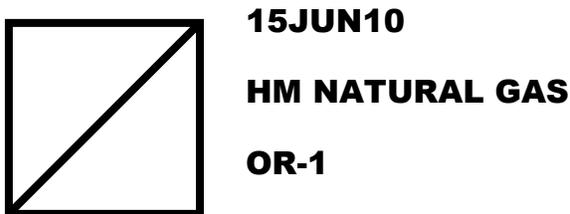
The above symbol means that entry is forbidden until the natural gas is turned off. Then the “HM NATURAL GAS” will be lined out and a new date put in. “OR-1” means Oregon Team 1 placed this symbol on the wall.
